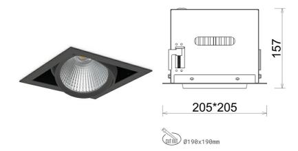
COB Light colour 4000 [K] | CRI Led chip flux 3122 [lm] Luminous flux 2497 [lm] System power 21 [W] Luminaire Efficiency 119 [lm/W] Beam angle 60° Controller ON/OFF MacAdam 3 SDCM
