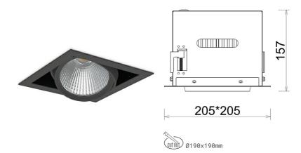
COB Light colour 3500 [K] | CRI Led chip flux 4453 [lm] Luminous flux 3562 [lm] System power 31 [W] Luminaire Efficiency 115 [lm/W] Beam angle 60° Controller ON/OFF MacAdam 3 SDCM
