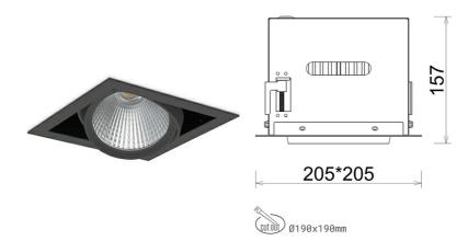
COB Light colour 3500 [K] | CRI Led chip flux 2783 [lm] Luminous flux 2226 [lm] System power 19 [W] Luminaire Efficiency 117 [lm/W] Beam angle 60° Controller ON/OFF MacAdam 3 SDCM
