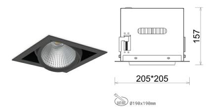
COB Light colour 3000 [K] | CRI Led chip flux 1905 [lm] Luminous flux 1524 [lm] System power 14 [W] Luminaire Efficiency 109 [lm/W] Beam angle 30° Controller ON/OFF MacAdam 3 SDCM
