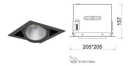
COB Light colour 2700 [K] | CRI Led chip flux 2963 [lm] Luminous flux 2370 [lm] System power 21 [W] Luminaire Efficiency 113 [lm/W] Beam angle 15° Controller ON/OFF MacAdam 3 SDCM
