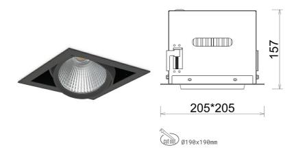
COB 3000 [K] CRI97 Light colour CRI Led chip flux 1144 [lm] Luminous flux 915 [lm] System power 10 [W] Luminaire Efficiency 92 [lm/W] 30° Beam angle Controller ON/OFF MacAdam 3 SDCM
