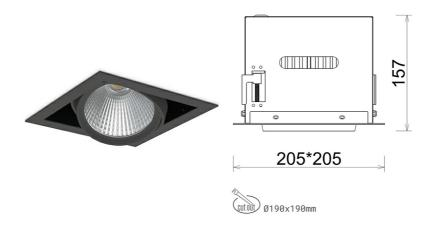
COB 5700 [K] SPECIAL Light colour CRI Led chip flux 3255 [lm] Luminous flux 2604 [lm] System power 25 [W] Luminaire Efficiency 104 [lm/W] Beam angle 45° Controller ON/OFF MacAdam 3 SDCM
