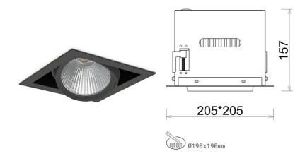
COB 4200 [K] MEAT WHITE Light colour CRI 90 Led chip flux 2519 [lm] Luminous flux 2015 [lm] System power 25 [W] Luminaire Efficiency 81 [lm/W] Beam angle 45° Controller ON/OFF MacAdam 3 SDCM
