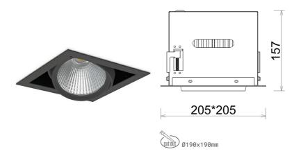
COB 4000 [K] HI EFFICIENT Light colour CRI 90 Led chip flux 5811 [lm] Luminous flux 4648 [lm] System power 36 [W] Luminaire Efficiency 129 [lm/W] Beam angle 60° Controller ON/OFF MacAdam 3 SDCM
