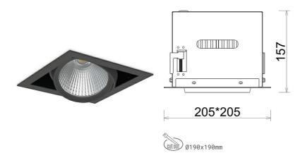
COB 4000 [K] HI EFFICIENT Light colour CRI 90 Led chip flux 1625 [lm] Luminous flux 1300 [lm] System power 10 [W] Luminaire Efficiency 130 [lm/W] Beam angle 45° Controller ON/OFF MacAdam 3 SDCM
