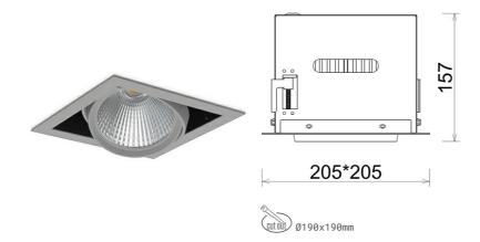
COB 2500 [K] BREAD Light colour CRI Led chip flux 3621 [lm] Luminous flux 2896 [lm] System power 31 [W] Luminaire Efficiency 93 [lm/W] Beam angle 45° Controller ON/OFF MacAdam 3 SDCM
