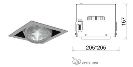
COB Light colour 4000 [K] | CRI Led chip flux 3383 [lm] Luminous flux 2706 [lm] System power 27 [W] Luminaire Efficiency 100 [lm/W] Beam angle 15° Controller ON/OFF MacAdam 3 SDCM
