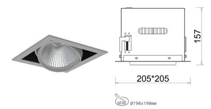
COB Light colour 5000 [K] | CRI Led chip flux 3475 [lm] Luminous flux 2780 [lm] System power 23 [W] Luminaire Efficiency 121 [lm/W] Beam angle 30° Controller ON/OFF MacAdam 3 SDCM
