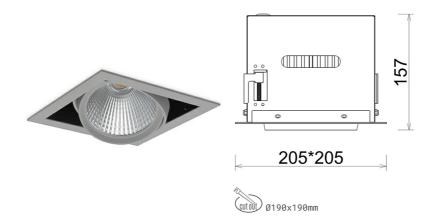
COB Light colour 5000 [K] | CRI Led chip flux 2895 [lm] Luminous flux 2316 [lm] System power 19 [W] Luminaire Efficiency 122 [lm/W] Beam angle 30° Controller ON/OFF MacAdam 3 SDCM
