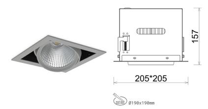
COB Light colour 3500 [K] | CRI Led chip flux 5010 [lm] Luminous flux 4008 [lm] System power 35 [W] Luminaire Efficiency 115 [lm/W] Beam angle 15° Controller ON/OFF MacAdam 3 SDCM
