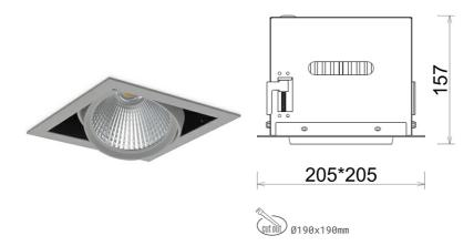
COB Light colour 3000 [K] | CRI Led chip flux 1361 [lm] Luminous flux 1088 [lm] System power 10 [W] Luminaire Efficiency 109 [lm/W] Beam angle 60° Controller ON/OFF MacAdam 3 SDCM
