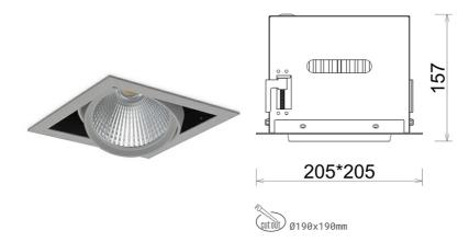
COB Light colour 2700 [K] | CRI Led chip flux 2963 [lm] Luminous flux 2370 [lm] System power 21 [W] Luminaire Efficiency 113 [lm/W] Beam angle 45° Controller ON/OFF MacAdam 3 SDCM
