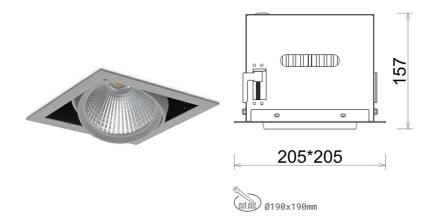
COB 3000 [K] CRI97 Light colour CRI Led chip flux 3735 [lm] Luminous flux 2988 [lm] System power 35 [W] Luminaire Efficiency 85 [lm/W] 60° Beam angle Controller ON/OFF MacAdam 3 SDCM
