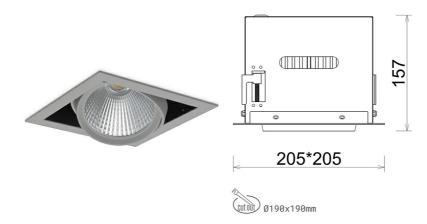
COB 4200 [K] MEAT WHITE Light colour CRI 90 Led chip flux 1412 [lm] Luminous flux 1129 [lm] System power 14 [W] Luminaire Efficiency 81 [lm/W] Beam angle 15° Controller ON/OFF MacAdam 3 SDCM
