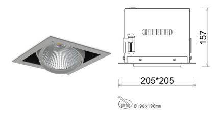
COB 4200 [K] MEAT WHITE Light colour CRI 90 Led chip flux Luminous flux 818 [lm] System power 10 [W] Luminaire Efficiency 82 [lm/W] Beam angle 15° Controller ON/OFF MacAdam
