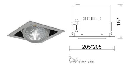
COB 4000 [K] HI EFFICIENT Light colour CRI 90 Led chip flux 5532 [lm] Luminous flux 4425 [lm] System power 34 [W] Luminaire Efficiency 130 [lm/W] Beam angle 45° Controller ON/OFF MacAdam 3 SDCM
