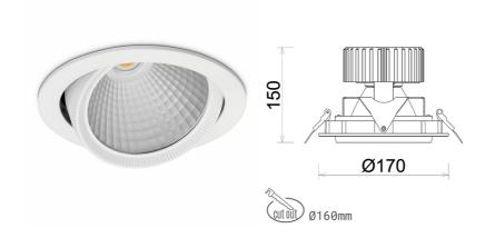
COB 2500 [K] BREAD Light colour CRI Led chip flux 3621 [lm] Luminous flux 2896 [lm] System power 31 [W] Luminaire Efficiency 93 [lm/W] Beam angle 30° Controller ON/OFF MacAdam 3 SDCM
