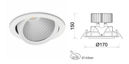
COB 2500 [K] BREAD Light colour CRI Led chip flux 3621 [lm] Luminous flux 2896 [lm] System power 31 [W] Luminaire Efficiency 93 [lm/W] Beam angle 15° Controller ON/OFF MacAdam 3 SDCM
