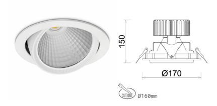
COB Light colour 4000 [K] | CRI Led chip flux 1208 [lm] Luminous flux 966 [lm] System power 10 [W] Luminaire Efficiency 97 [lm/W] Beam angle 45° Controller ON/OFF MacAdam 3 SDCM
