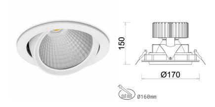
COB Light colour 4000 [K] | CRI Led chip flux 4350 [lm] Luminous flux 3480 [lm] System power 35 [W] Luminaire Efficiency 99 [lm/W] Beam angle 15° Controller ON/OFF MacAdam 3 SDCM
