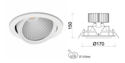
COB Light colour 3000 [K] | CRI Led chip flux 2305 [lm] Luminous flux 1844 [lm] System power 19 [W] Luminaire Efficiency 97 [lm/W] Beam angle 45° Controller ON/OFF MacAdam 3 SDCM
