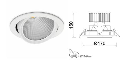
COB Light colour 2700 [K] | CRI Led chip flux 2667 [lm] Luminous flux 2133 [lm] System power 23 [W] Luminaire Efficiency 93 [lm/W] Beam angle 45° Controller ON/OFF MacAdam 3 SDCM
