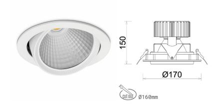
COB Light colour 2700 [K] | CRI Led chip flux 3555 [lm] Luminous flux 2844 [lm] System power 31 [W] Luminaire Efficiency 92 [lm/W] 30° Beam angle Controller ON/OFF MacAdam 3 SDCM
