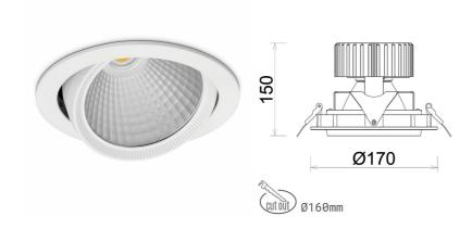
COB Light colour 2700 [K] | CRI Led chip flux 2888 [lm] Luminous flux 2310 [lm] System power 25 [W] Luminaire Efficiency 92 [lm/W] 30° Beam angle Controller ON/OFF MacAdam 3 SDCM
