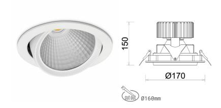
COB Light colour 2700 [K] | CRI Led chip flux 1111 [lm] Luminous flux 888 [lm] System power 10 [W] Luminaire Efficiency 89 [lm/W] Beam angle 15° Controller ON/OFF MacAdam 3 SDCM
