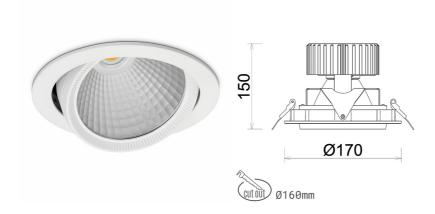
COB Light colour 5000 [K] | CRI Led chip flux 1447 [lm] Luminous flux 1157 [lm] System power 10 [W] Luminaire Efficiency 116 [lm/W] Beam angle 60° Controller ON/OFF MacAdam 3 SDCM
