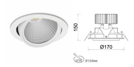
COB Light colour 5000 [K] | CRI Led chip flux 4633 [lm] Luminous flux 3706 [lm] System power 31 [W] Luminaire Efficiency 120 [lm/W] Beam angle 30° Controller ON/OFF MacAdam 3 SDCM
