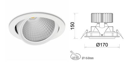
COB Light colour 5000 [K] | CRI Led chip flux 3475 [lm] Luminous flux 2780 [lm] System power 23 [W] Luminaire Efficiency 121 [lm/W] Beam angle 30° Controller ON/OFF MacAdam 3 SDCM
