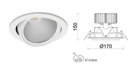
COB Light colour 5000 [K] | CRI Led chip flux 2027 [lm] Luminous flux 1621 [lm] System power 14 [W] Luminaire Efficiency 116 [lm/W] Beam angle 30° Controller ON/OFF MacAdam 3 SDCM
