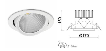
COB Light colour 4000 [K] | CRI Led chip flux 1987 [lm] Luminous flux 1589 [lm] System power 14 [W] Luminaire Efficiency 114 [lm/W] Beam angle 30° Controller ON/OFF MacAdam 3 SDCM
