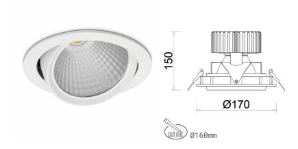
COB Light colour 4000 [K] | CRI Led chip flux 5110 [lm] Luminous flux 4088 [lm] System power 35 [W] Luminaire Efficiency 117 [lm/W] Beam angle 15° Controller ON/OFF MacAdam 3 SDCM
