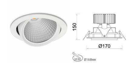
COB Light colour 3500 [K] | CRI Led chip flux 3061 [lm] Luminous flux 2448 [lm] System power 21 [W] Luminaire Efficiency 117 [lm/W] Beam angle 60° Controller ON/OFF MacAdam 3 SDCM
