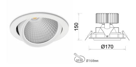
COB Light colour 3500 [K] | CRI Led chip flux 4453 [lm] Luminous flux 3562 [lm] System power 31 [W] Luminaire Efficiency 115 [lm/W] Beam angle 45° Controller ON/OFF MacAdam 3 SDCM
