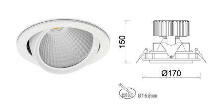
COB Light colour 3500 [K] | CRI Led chip flux 3061 [lm] Luminous flux 2448 [lm] System power 21 [W] Luminaire Efficiency 117 [lm/W] Beam angle 45° Controller ON/OFF MacAdam 3 SDCM
