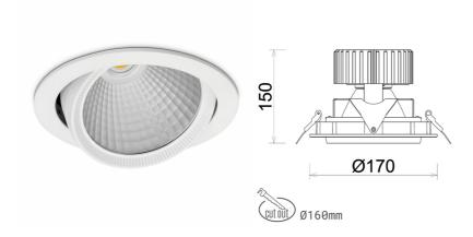
COB Light colour 3500 [K] | CRI Led chip flux 5010 [lm] Luminous flux 4008 [lm] System power 35 [W] Luminaire Efficiency 115 [lm/W] Beam angle 30° Controller ON/OFF MacAdam 3 SDCM
