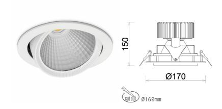
COB Light colour 3500 [K] | CRI Led chip flux 3618 [lm] Luminous flux 2894 [lm] System power 25 [W] Luminaire Efficiency 116 [lm/W] Beam angle 30° Controller ON/OFF MacAdam 3 SDCM
