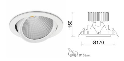
COB Light colour 3500 [K] | CRI Led chip flux 1391 [lm] Luminous flux 1112 [lm] System power 10 [W] Luminaire Efficiency 111 [lm/W] Beam angle 15° Controller ON/OFF MacAdam 3 SDCM
