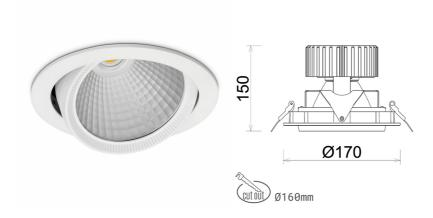
COB Light colour 3000 [K] | CRI Led chip flux 2722 [lm] Luminous flux 2177 [lm] System power 19 [W] Luminaire Efficiency 115 [lm/W] Beam angle 60° Controller ON/OFF MacAdam 3 SDCM
