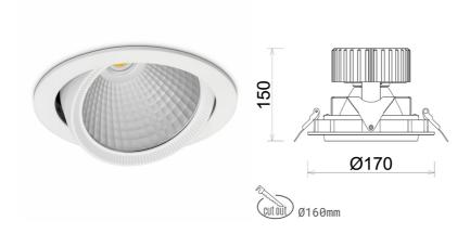
COB Light colour 2700 [K] | CRI Led chip flux 5119 [lm] Luminous flux 4095 [lm] System power 37 [W] Luminaire Efficiency 111 [lm/W] Beam angle 60° Controller ON/OFF MacAdam 3 SDCM
