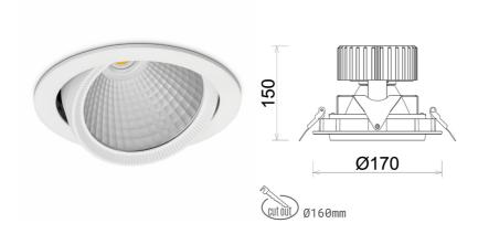
COB Light colour 2700 [K] | CRI Led chip flux 3772 [lm] Luminous flux 3017 [lm] System power 27 [W] Luminaire Efficiency 112 [lm/W] Beam angle 30° Controller ON/OFF MacAdam 3 SDCM
