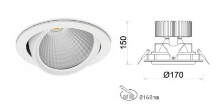
COB Light colour 2700 [K] | CRI Led chip flux 3233 [lm] Luminous flux 2586 [lm] System power 23 [W] Luminaire Efficiency 112 [lm/W] Beam angle 30° Controller ON/OFF MacAdam 3 SDCM
