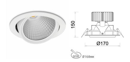
COB Light colour 2700 [K] | CRI Led chip flux 2963 [lm] Luminous flux 2370 [lm] System power 21 [W] Luminaire Efficiency 113 [lm/W] Beam angle 30° Controller ON/OFF MacAdam 3 SDCM
