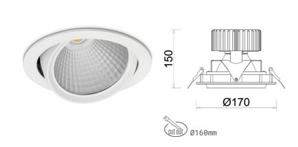
COB Light colour 2700 [K] | CRI Led chip flux 2694 [lm] Luminous flux 2155 [lm] System power 19 [W] Luminaire Efficiency 113 [lm/W] Beam angle 15° Controller ON/OFF MacAdam 3 SDCM
