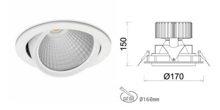
COB Light colour 2700 [K] | CRI Led chip flux 1347 [lm] Luminous flux 1077 [lm] System power 10 [W] Luminaire Efficiency 108 [lm/W] Beam angle 15° Controller ON/OFF MacAdam 3 SDCM
