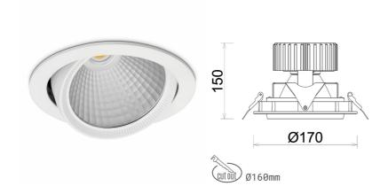
COB 3000 [K] CRI97 Light colour CRI Led chip flux 3735 [lm] Luminous flux 2988 [lm] System power 35 [W] Luminaire Efficiency 85 [lm/W] Beam angle 45° Controller ON/OFF MacAdam 3 SDCM
